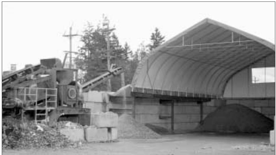
*A crusher turns glass bottles into fine particles for use in a wide range of applications.*
